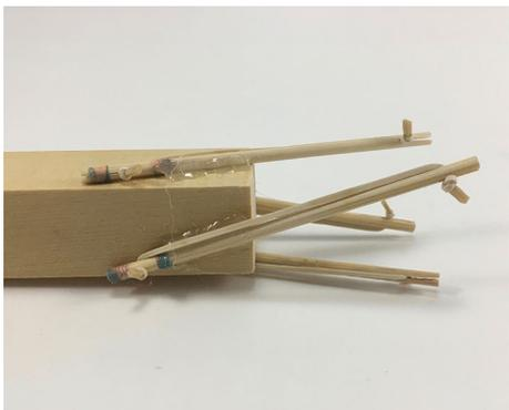
**Fig. 45** Hard transitional region. Spiral tensegrity mast
