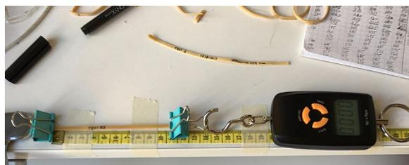
**Fig. 56** Rubber band test setup
