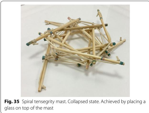
**Fig. 35** Spiral tensegrity mast. Collapsed state. Achieved by placing a glass on top of the mast
