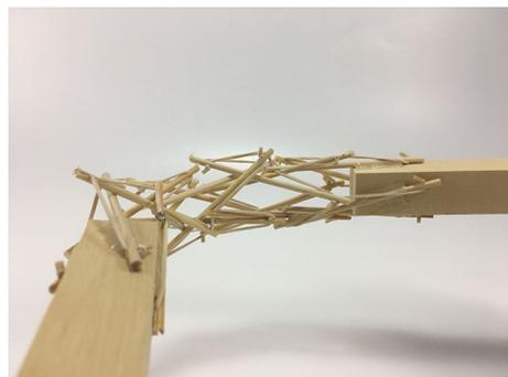
**Fig. 47** Hard transitional region prototype. Spiral tensegrity mast
