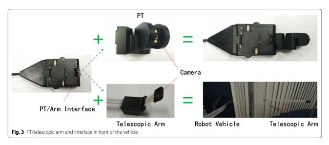
generator. Made of flexible material, the telescopic arm can be put in the tubes. The center of the telescopic arm contains many holes, so it could be fixed and moved by motor. A camera in front of the telescopic arm allows transfer of video for checking tubes and further analysis.
