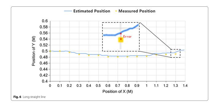
error is considered as the difference between yellow point and the point at which the blue line intersects the datum line of X axis. The range of the vehicle's regular activity is at a height about 1 m, and the width of the vehicle is 0.12 m. We consider the error that below half of the vehicle's width is acceptable, which is 6%.
